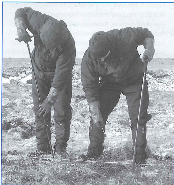
Figure 8 Probing of the soil to locate buried objects in a remote location in Eastern Europe (after Donnelly & Harrison 2010a).
