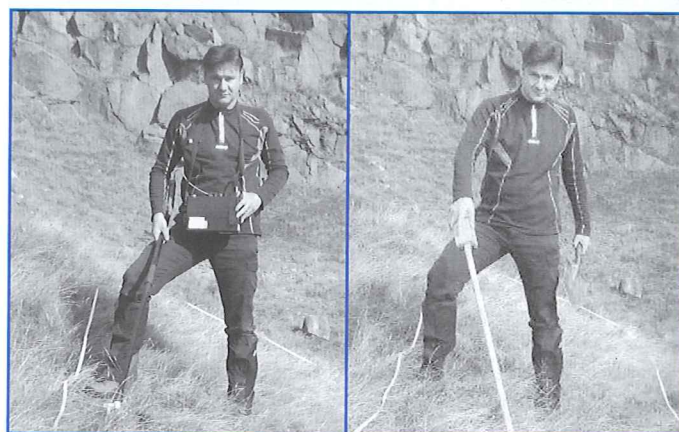
Figure 10 Forensic Geologist, Dr Laurance Donnelly, conducting a geophysical survey (electromagnetic) to search and locate a murder victim's grave in Europe (after Donnelly 2010)
