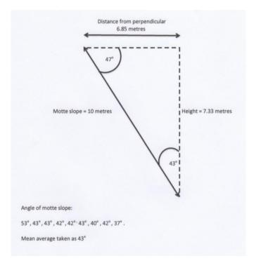
Figure 06: Motte Slope Calculation
