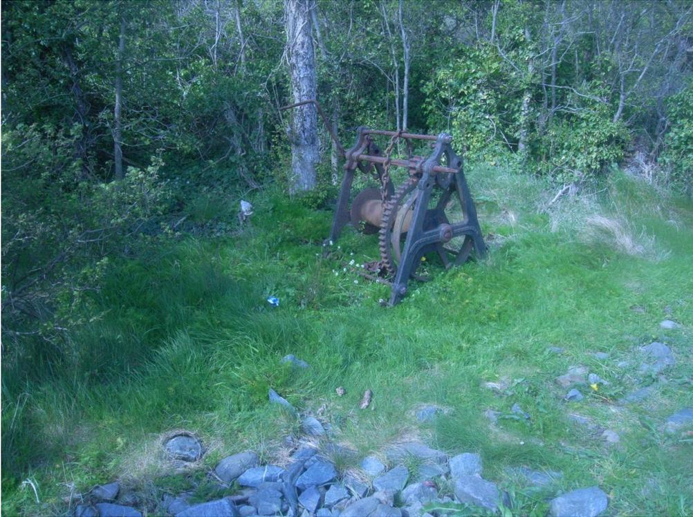
Figure 49: Old winch for recovering boats, at the head of the Slipway
