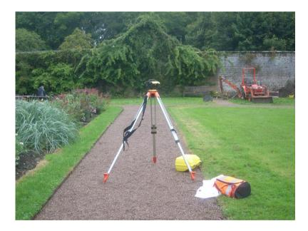
Figure 06: Leica Sprinter electronic measuring device in position during the survey
